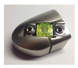
The washers are then placed on top of the fuse with the crown of the washer pointed up.
